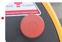
Emergency Power-off Switch
