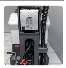
Easy access and handling to clean recovery tank and floater. Less downtimes due to simple maintenance and construction Great visibility and cleaning capability on hard to reach edges on both sides of the brush.
