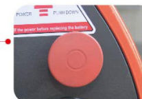
Emergency Power-off Switch
