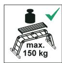
Max. load of platform in scaffold position (see EN 131-4:2007, Clause 7) declared by the manufacturer (120 kg to 150 kg) (only if necessary due to design of ladder).
