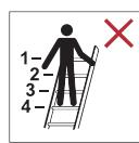
Do not climb above the rung or tread recommended by the producer, of a combination ladder used in the standing ladder position, with extending ladder at the top or in the stairway position. The minimum requirement shall always be: Do not climb above the top four steps/rungs.
