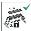
If the ladder is used as a platform, only deckings recommended by the ladder producer shall be used. The decking shall be secured before use (only if necessary due to design of ladder).
