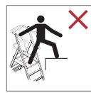
Do not step off the side of the mobile platform ladder onto another surface.
