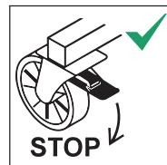
Lock the wheels while using the ladder.
