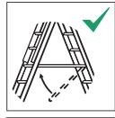
Use the ladder with restraint devices engaged only (only if necessary due to design of ladder).
