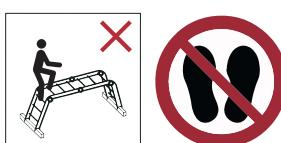
Do not use the ladder at platform position , without decking component.
